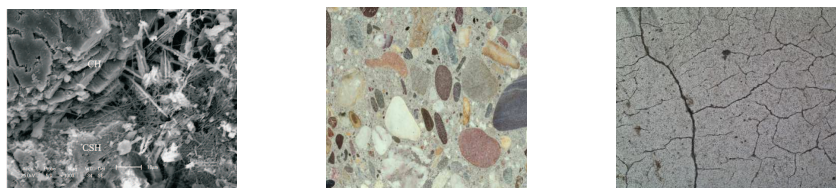
Figure 1: Concrete structure on the nano-, micro- and macro-scale
